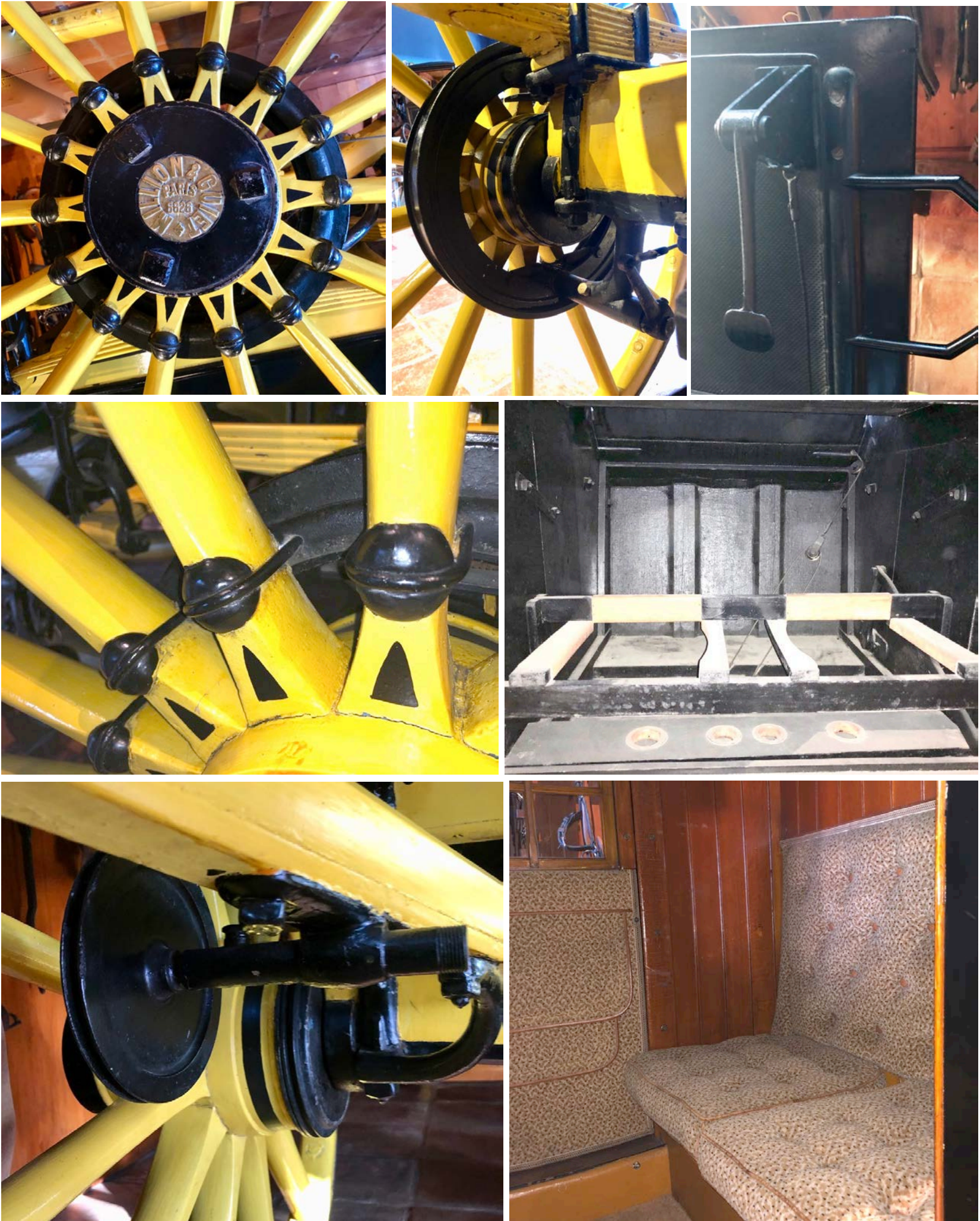
129 Details on the Private Road-Coach EB 16 standing in Portugal: brake system, parts of the odometer and the interior lining.
