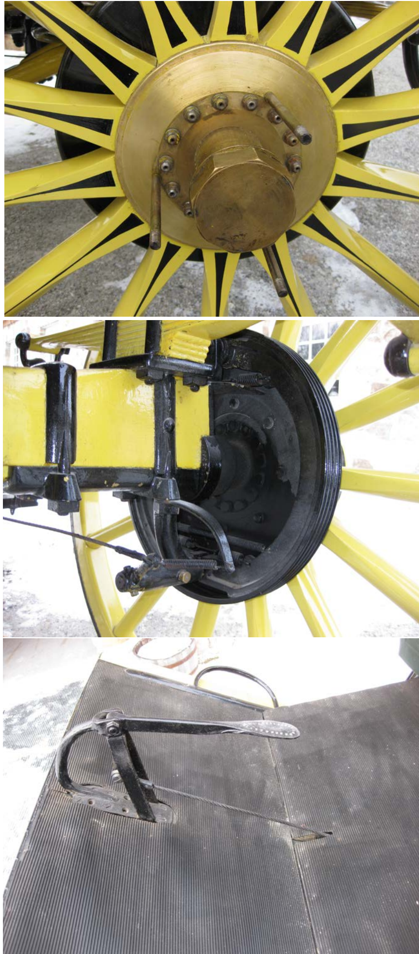
59 (EB 01) The construction of the hub and brake on the Chariot-Coach. Top: The inner construction of the hub; Molsheim's pattern. Middle: The drum brake and cable. Bottom: Brake pedal on the footboard.
